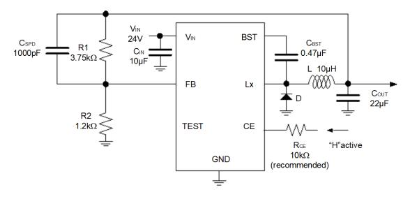
R1245x00xC/D Typical Application Circuit, 500 kHz,  $V_{OUT}$  = 3.3 V,  $V_{IN}$  = 24 V
