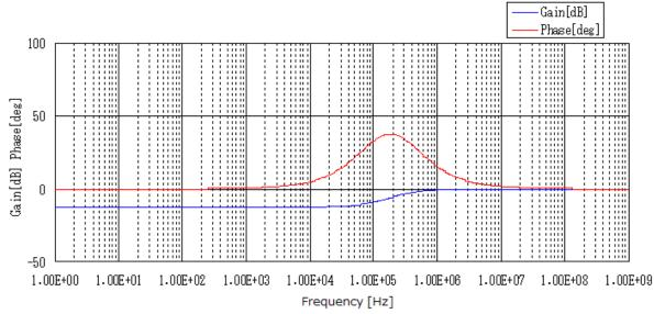
Figure 3. Transfer function BODE plot from V<sub>OUT</sub> to FB (R1=3.75kΩ, R2=1.2kΩ, Cspd=470pF)
