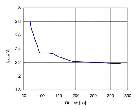
Figure 6. On time and Lx current limit, Lx pin current peak value ILXLIM
