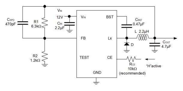
R1245x00xG/H Typical Application Circuit, 2400 kHz,  $V_{\text{OUT}}$  = 5. 0 V,  $V_{\text{IN}}$  = 12 V
